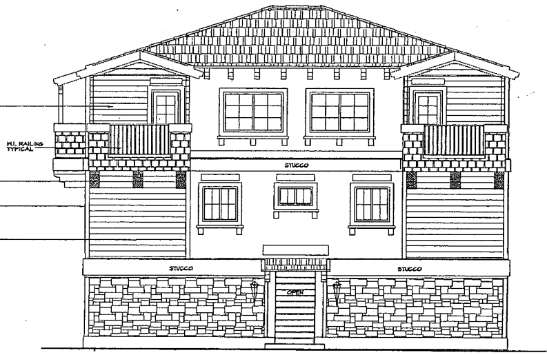
TYPICAL REAR ELEVATION TYPE "A" UNIT 1/4" = 1'-0"
