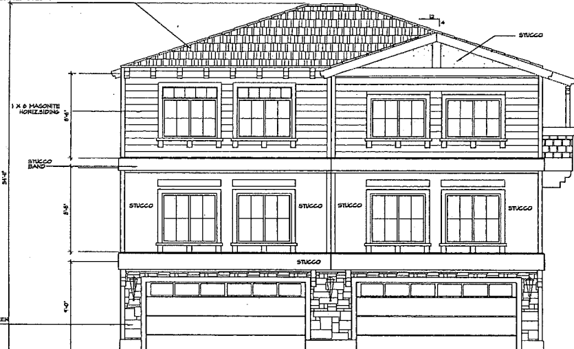
TYPICAL STREET ELEVATION BUILDING "A" 1/4" = 1'-0"
