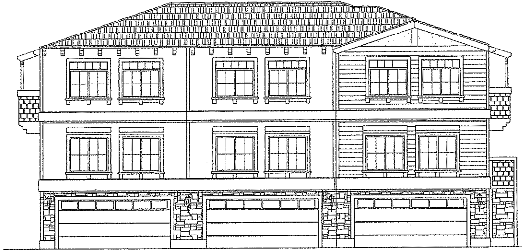
TYPICAL STREET ELEVATION ISLAND TRIPLEX
