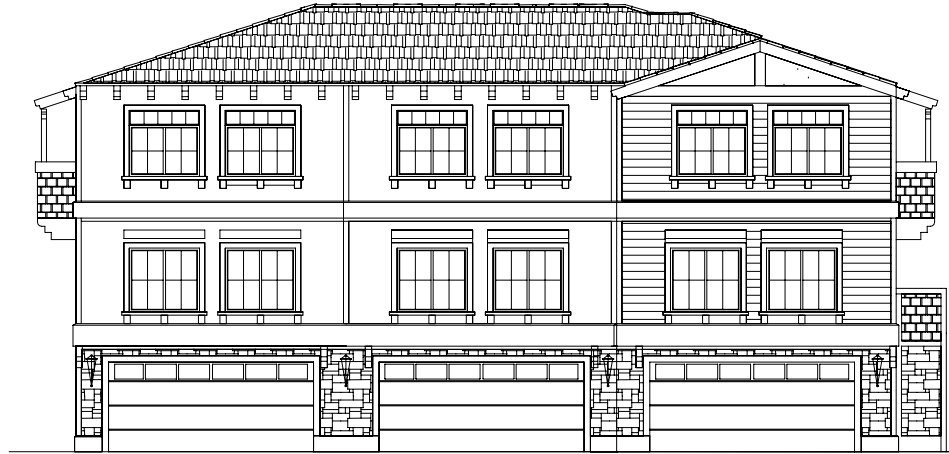
TYPICAL STREET ELEVATION ISLAND TRIPLEX
