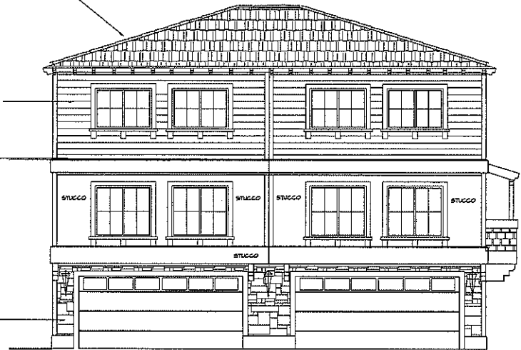
TYPICAL STREET ELEVATION BUILDING "A" 1/4" = 1'-0"
