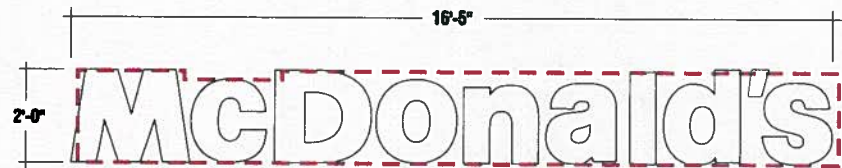
A2 LED ILLUMINATED CHANNEL LETTERS Quantity: One (1) Required 32.4 Sq. Ft. Scale: 3/8" = 1'-0"
