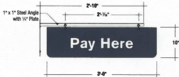
E SINGLE FACE NON-ILLUMINATED WINDOW POSITION PANEL W/MOUNTING BRACKET 2.49 Sq. Ft. Quantity: One (1) Required Scale: 1" = 1'-0"
