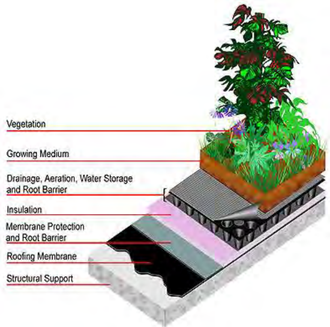
Figure E-8. Green Roof Schematic
