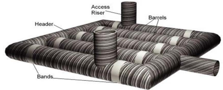
TYPICAL INSTALLATION (FOR COVER DEPTHS UP TO 75% OF MAX ALLOWABLE COVER) (< 2.0' FROM TOP OF PAVEMENT TO TOP OF PIPE)
