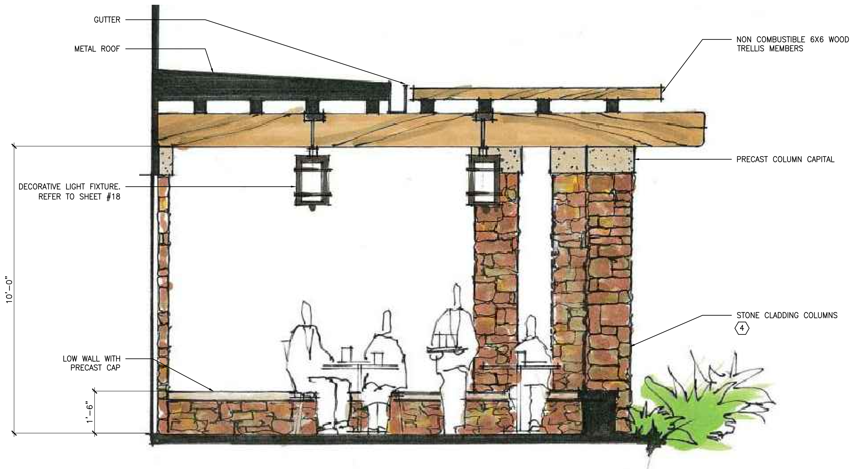
1 OUTDOOR DINING AREA SECTION / ELEVATION
