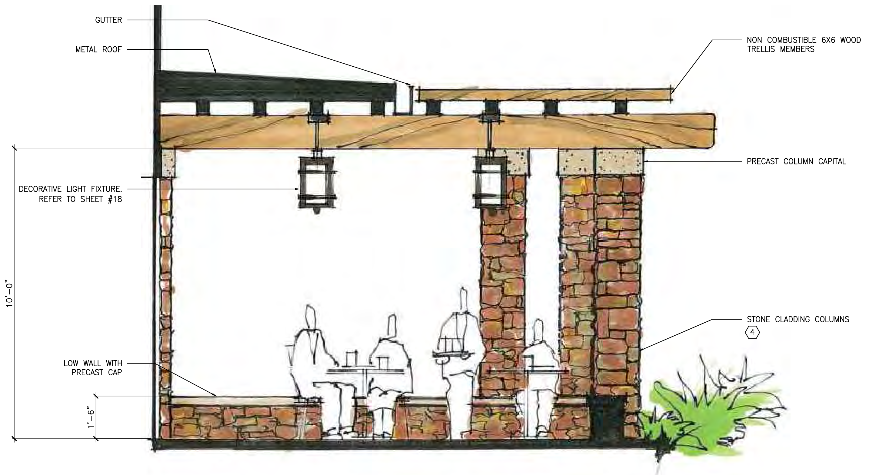
1 OUTDOOR DINING AREA SECTION / ELEVATION
