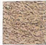
Sandblasted Concrete 1-E
