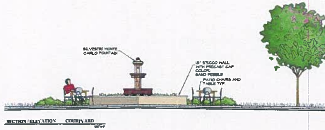
SECTION ELEVATION COURTYARD 1/4" = 1'-0"
