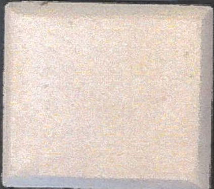
SMOOTH COAT PLASTER
