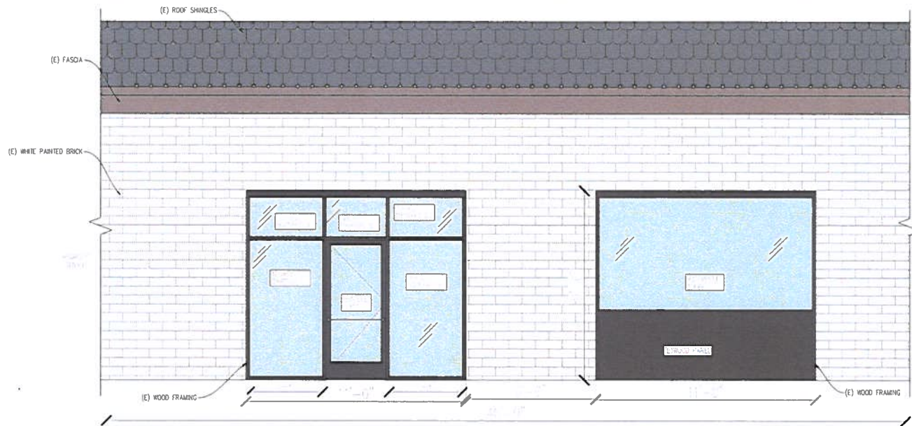
1 RESTAURANT FRONT ELEVATION A-2.1 SCALE: 1/2" = 1'-0"
