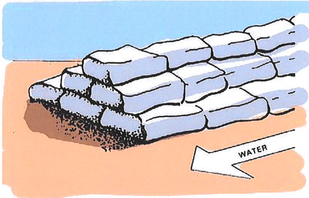
Figure 11: Sandbag Stacking – Allow for a wider sand bag wall when stacking sand bags higher.
