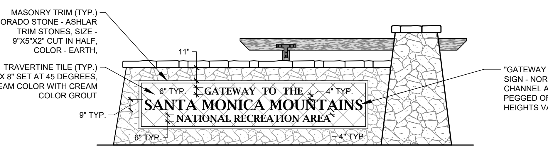
ELEVATION - WEST SIDE (SOUTH FACE)
