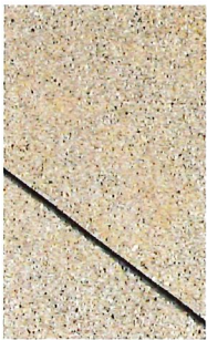
DRIVEWAY/ACCESS ROAD SAND FINISH CONCRETE COLOR: TAN
