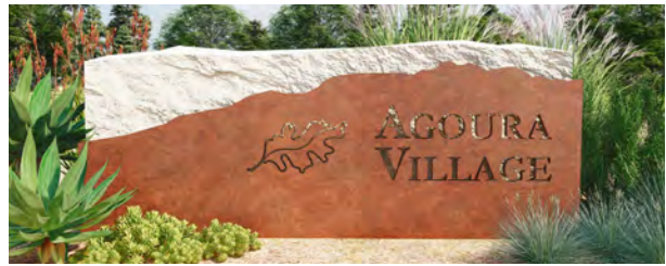
Village Gateway Monument - Concept 1 - sandstone wall with corten steel silhouette of Ladyface Mountain and laser cut logo and typology.
